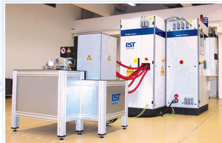
EMPT manufacturing system of PSTproducts
